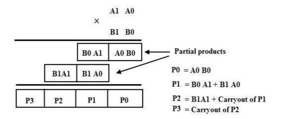
The first partial product is obtained by the AND gate which is nothing but a least significant bit of the multiplication result. Since the second partial product is shifted to the left position, the first partial second term and second partial product first term is added by half adder and produce the sum output along with the carry out.
