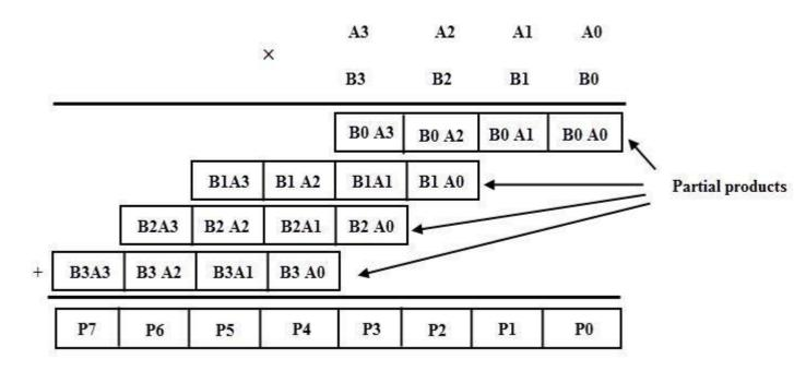
The logic circuit for the  $4 \times 4$  binary multiplication can be implemented by using three binary full adders along with AND gates.
