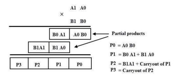
This process involves the multiplication of two digits and the addition of digits with or without carry. After the multiplication of each bit to the multiplicand, partial products are generated, and then these products are added to produce the total sum which represents the binary multiplication value.
